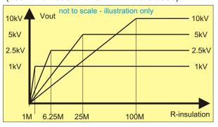
For the **6200IN and 6201IN** instruments, the insulation resistance higher than 454M will give best result (when 10kV selected), specially due to the current limit being a little different from one instrument to an other one. Accuracy will be worse if you read less than a total of 454M (227M on each if two H.V.I.M. are used)
